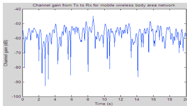
Fig.5. Analysis of Channel gain Vs Time using SISO
